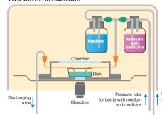
\*Syringe pump or peristaltic pump is necessary to pressurize the solution bottles.
